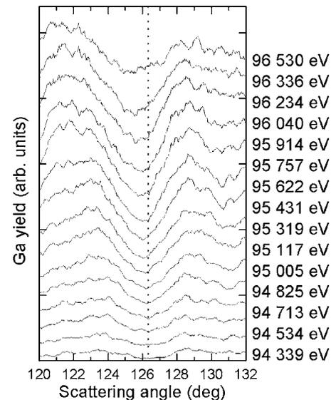
FIG. 2. MEIS angular spectra of the uncapped GaN QDs layer taken for different energies ranging from 96 530 eV (surface of the GaN QD) to 94 339 eV (AlN/GaN interface). The dotted line shows the blocking dip corresponding to the AlN/GaN interface. Note a satellite dip at  $126.8^\circ$  for the 96 530 eV line, which is assigned to the presence of the wetting layer.
