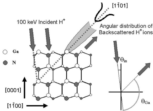
FIG. 1. Scheme of the scattering geometry in the  $(11\bar{2}0)$  plane for medium ion energy scattering experiments.
