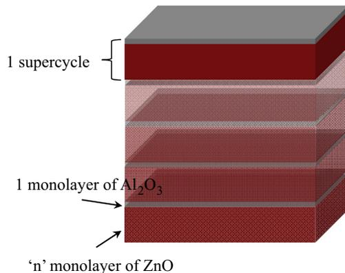
Fig. 1. Schematic diagram of Al-doped ZnO film stack to fabricated with various Al doping concentration by ALD.
