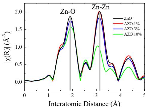
Fig. 3. Fourier transformed EXAFS data of Al-doped ZnO as a function of Al doping concentration, obtained by Zn K edge spectra.
