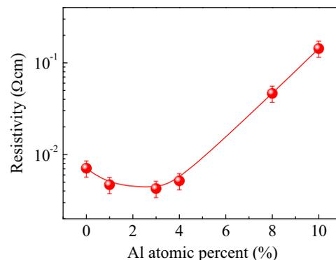
Fig. 2. Resistivity of Al-doped ZnO films as a function of Al doping concentration.
