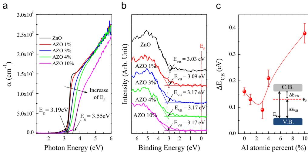
Fig. 5. (a) Absorption coefficient spectra, (b) valence spectra, and (c) conduction band offset ( $\Delta E_{CB}$ ) between minimum of conduction band and Fermi level of Al-doped ZnO films as a function of Al doping concentration.
