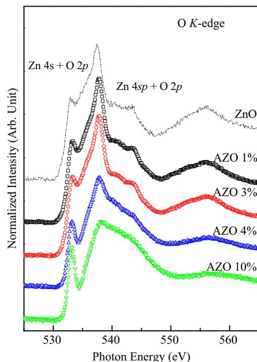
Fig. 4. O K edge spectra of Al-doped ZnO films as a function of Al doping concentration.
