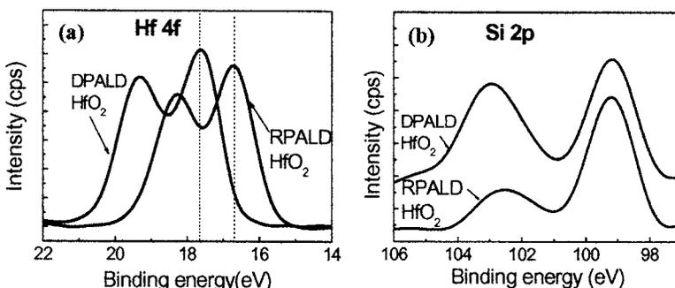
FIG. 3. XPS spectra of as-grown RPALD and DPALD samples showing (a) the Hf  $4f$  and (b) Si  $2p$  peaks. The  $\text{HfO}_2$  films of the samples were grown using 50 ALD cycles and the plasma power of 100 W.
