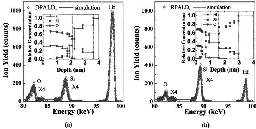
FIG. 4. MEIS results for (a) as-grown DPALD and (b) RPALD  $\text{HfO}_2$  films. The open circles and solid lines represent raw data and fitted data, respectively. The inset shows the relative concentration along the depth direction of the films calculated from the fitted results.
