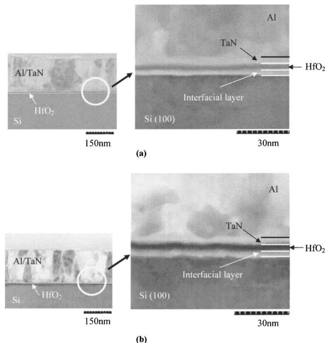
FIG. 6. Cross-sectional TEM micrographs of replacement Al/TaN-gate nMOSFETs with HfO<sub>2</sub> gate dielectrics grown using (a) the RPALD and (b) the DPALD methods. The effective width and length of the two nMOSFETs were about 10.0  $\mu\text{m}$ .
