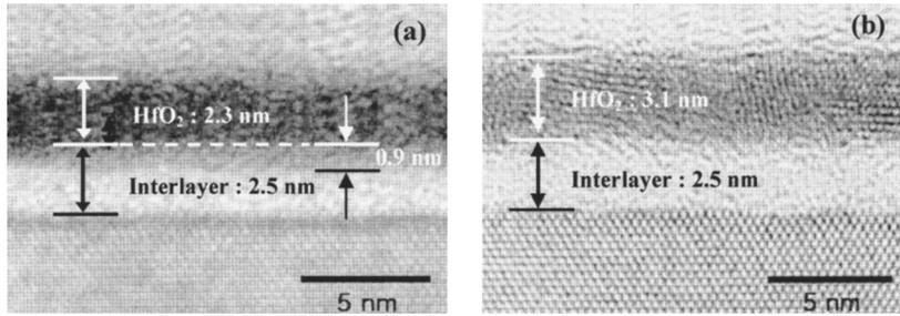
FIG. 2. A cross-sectional HRTEM micrograph of as-grown  $\text{HfO}_2$  films deposited on a Si substrate using (a) the RPALD and (b) the DPALD methods at a deposition temperature of 250 °C using  $\text{Hf}(\text{NEt}_2)_4$  precursor.
