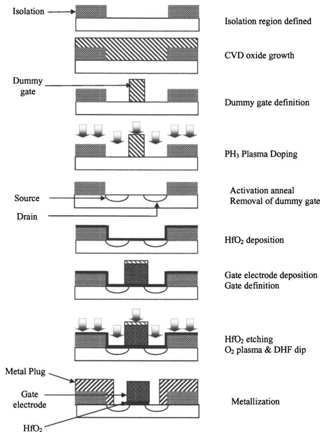
FIG. 1. The replacement gate nMOSFET fabrication process.
