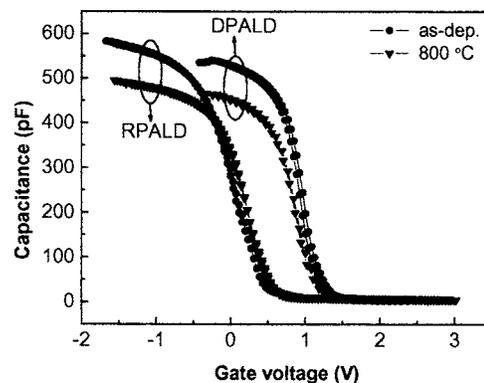
FIG. 5. Capacitance-voltage ( $C$ - $V$ ) curves for as-grown and annealed  $\text{HfO}_2$  films deposited using the RPALD and DPALD methods.
