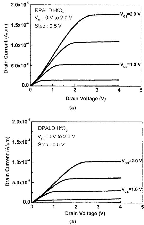
FIG. 8. Drain current vs drain voltage curves of Al/TaN replacement gate nMOSFETs with HfO<sub>2</sub> gate dielectrics grown using (a) the RPALD and (b) the DPALD methods.  $V=0$  to 2.0 V. Step=0.5 V.
