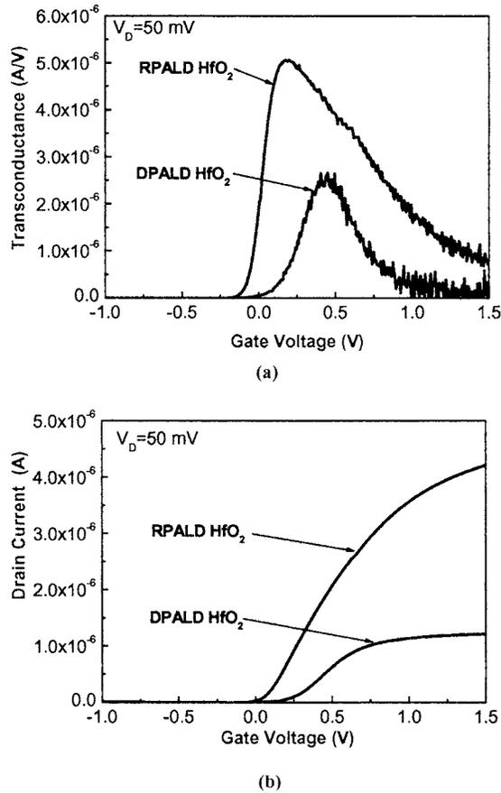
FIG. 7. The transconductance vs gate voltage ( $G_m$ - $V_g$ ) and drain current vs gate voltage curves ( $I_d$ - $V_g$ ) of replacement Al/TaN-gate nMOSFETs with HfO<sub>2</sub> gate dielectrics.
