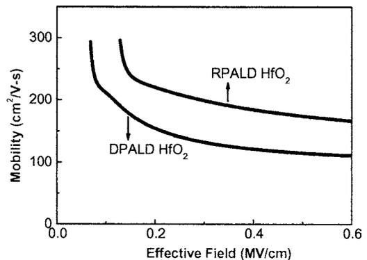
FIG. 9. Effective mobility as a function of effective electric field for replacement Al/TaN-gate nMOSFETs with HfO<sub>2</sub> gate dielectrics.
