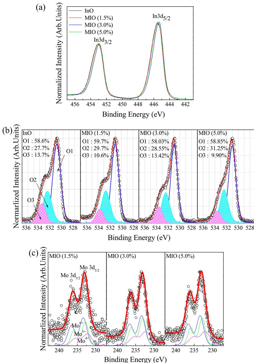
Fig. 2. XPS spectra of indium oxide films for (a) In 3d, (b) O 1s, and (c) Mo 3d of MIO films as a function of Mo doping concentration. O 1s and Mo 3d in (b) and (c) were deconvoluted with sub-chemical bonding states.
