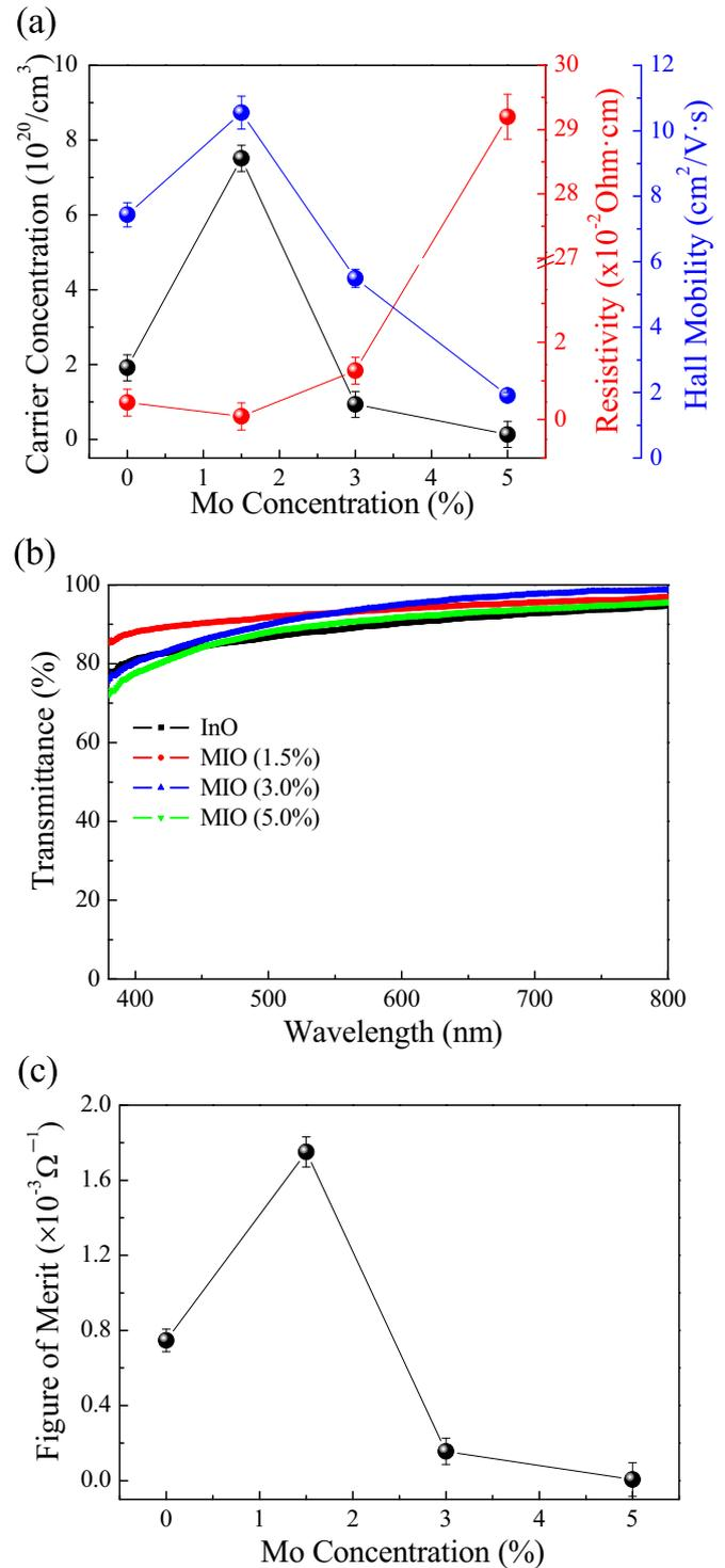
**Fig. 1.** (a) Electrical properties, including carrier concentration, Hall mobility, and resistivity of MIO films, (b) optical transmittance spectra, and (c) figure of merit (FOM) value as a function of Mo doping concentration.
