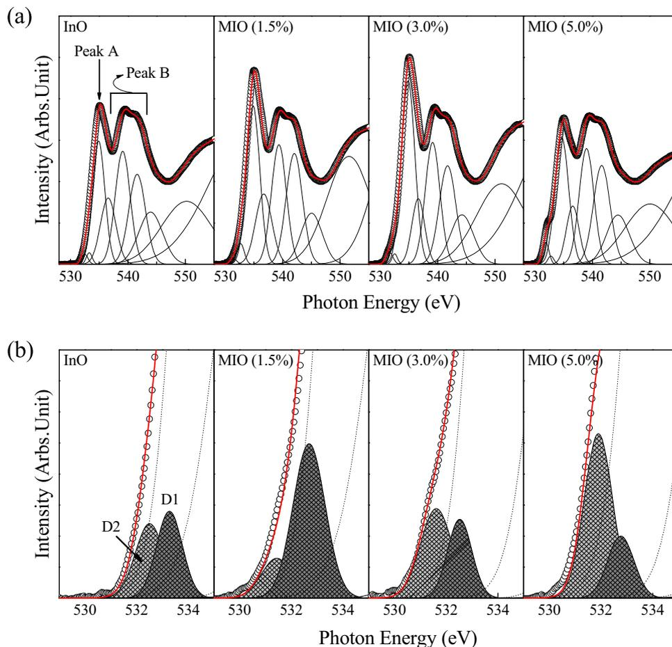
**Fig. 3.** (a) Normalized XAS O K edge spectra, and Gaussian fits of normalized XAS O K edge spectra, and (b) band edge states below the conduction band, as a function of Mo doping concentration.
