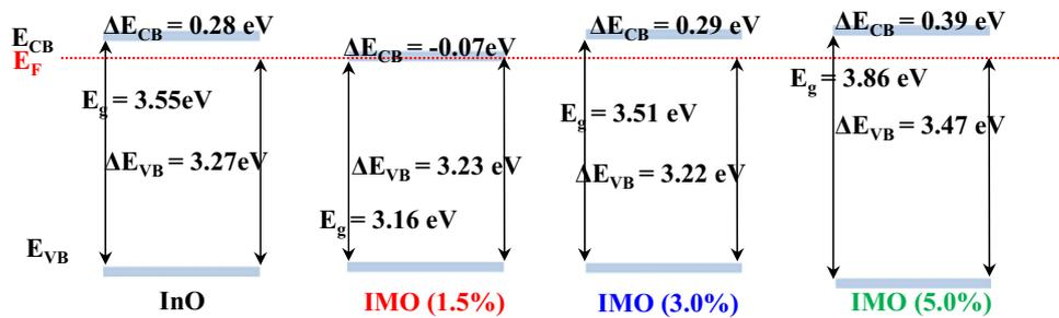
**Fig. 4.** Schematic energy level diagram, reflecting the relative energy position of the Fermi level ( $E_F$ ) with respect to the conduction band ( $E_{CB}$ ) minimum and valence band ( $E_{VB}$ ) maximum, as a function of Mo doping concentration.
