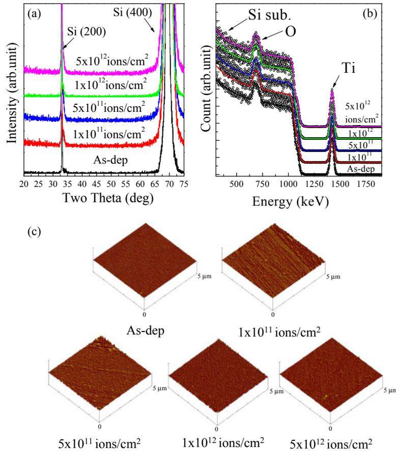
**Fig. 3.** (Color online) (a) XRD patterns, (b) RBS spectra, and (c) surface morphology using AFM for the as-deposited and irradiated  $\text{TiO}_{2-x}$  films as a function of Au ion irradiation dose.
