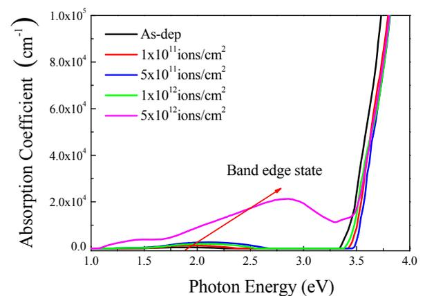
**Fig. 5.** (Color online) Absorption coefficient of the as-deposited and irradiated  $\text{TiO}_{2-x}$  films as a function of Au ion irradiation dose.
