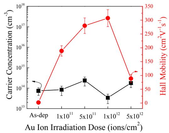
**Fig. 2.** (Color online) Electrical properties, including carrier concentration, and mobility for as-deposited and irradiated TiO<sub>2-x</sub> films as a function of Au ion irradiation dose.
