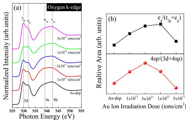
**Fig. 4.** (Color online) (a) Normalized O K-edge XAS spectra, (b) relative  $e_g/(e_g + t_{2g})$  states ratio of Ti 3d and relative  $4sp/(3d + 4sp)$  molecular orbital ratio of calculated by the Gaussian fitting results as a function of Au ion irradiation dose.
