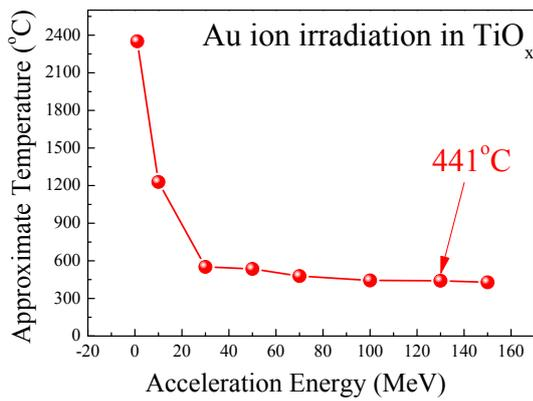
**Fig. 1.** (Color online) Approximate calculation of process temperature as a function of Au ion acceleration energy.
