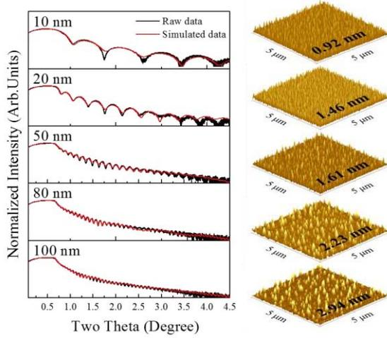
Fig. 3. Physical properties of WIZO film and interface layer at the WIZO–SiO<sub>2</sub> include film thickness, density, and interface/surface roughness.
