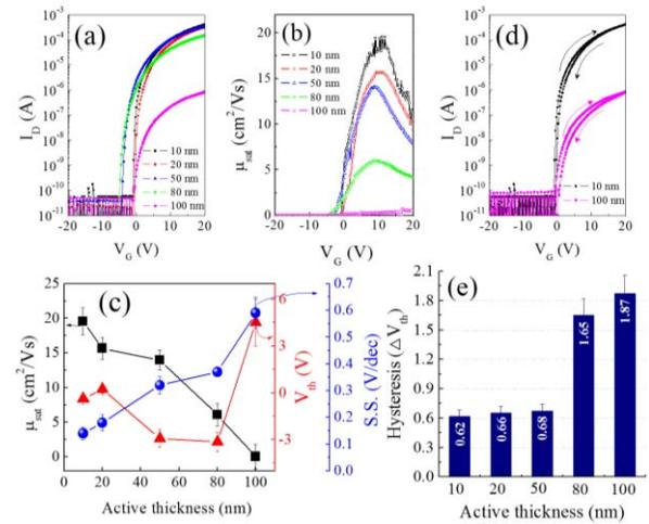
**Fig. 2.** (a) Transfer characteristics. (b) Calculated saturation mobility. (c) Clockwise hysteresis behaviors. (d) Extracted electrical parameters, namely the saturation mobility ( $\mu_{sat}$ ), threshold voltage ( $V_{th}$ ), and SS. (e) Variation of  $V_{th}$  with the hysteresis.
