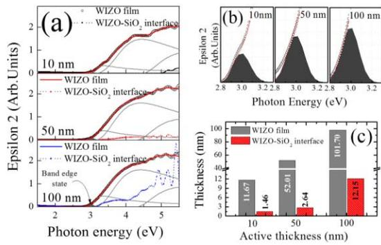
Fig. 4. (a) Imaginary part of the dielectric function ( $\epsilon_2$ ) spectra, (b) enlargements of the  $\epsilon_2$  spectra below the conduction band of the WIZO film with different film thicknesses. (c) Thickness of WIZO film and WIZO-SiO<sub>2</sub> interface.
