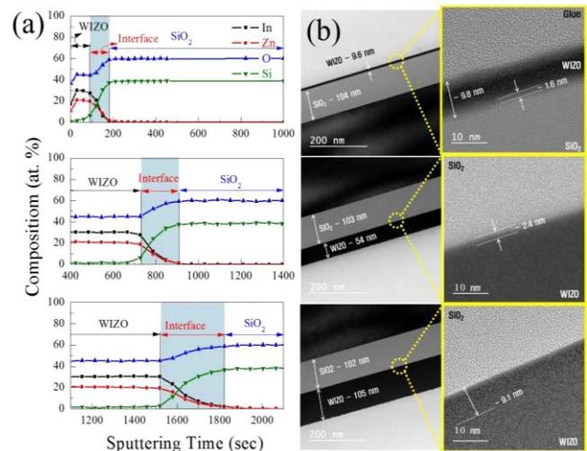
Fig. 5. Interface layer thickness between the SiO<sub>2</sub> and the WIZO as a function of film thickness studied by (a) XPS depth profiles and (b) cross-sectional TEM images.
