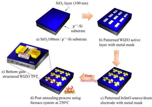
**Fig. 1.** Schematic illustration of overall bottom-gate structured WIZO TFT fabrication. (a) SiO<sub>2</sub>/p<sup>++</sup>-Si substrate, (b) WIZO deposition with a pattern by RF sputtering with various active layer thickness, (c) patterned ITO as a source/drain electrode, (d) postannealing process using furnace system at 250 °C in ambient air for 1 h, (e) bottom-gate structure WIZO TFT with channel width and length of 800 and 200 μm.
