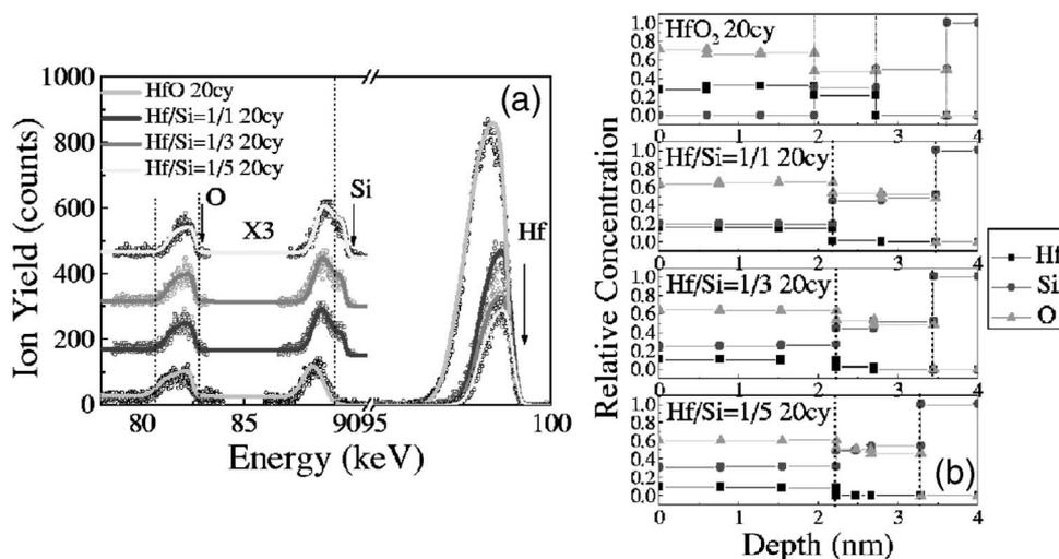
**Figure 1.** (a) MEIS energy spectra of Hf silicate-like films as a function of the ratio of alternate deposition cycles between  $\text{HfO}_2$  and  $\text{SiO}_2$  ( $\text{Hf/Si}$ );  $\text{Hf/Si} = 1/n$  ( $n = 1, 3, \text{ and } 5$ ). To equalize the quantities of Hf supplied, the total feeding cycles of Hf were fixed at 20 cycles. (b) Compositional depth profiles corresponding to Fig. 1a.
