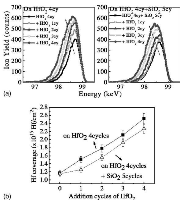
**Figure 3.** (a) The in situ MEIS energy spectra in the Hf region depending on the initial surface conditions as a function of additional HfO<sub>2</sub> cycles (4 cycles of HfO<sub>2</sub> and 4 cycles of HfO<sub>2</sub> + 5 cycles of SiO<sub>2</sub>). (b) The comparison of the calculated Hf coverage depending on the initial surface conditions as a function of additional HfO<sub>2</sub> cycles (4 cycles of HfO<sub>2</sub> and 4 cycles of HfO<sub>2</sub> + 5 cycles of SiO<sub>2</sub>).
