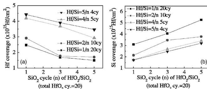
**Figure 2.** (a) Calculated Hf coverage depending on the ratio of  $\text{SiO}_2$  cycle. (b) Calculated Si coverage depending on the ratio of  $\text{SiO}_2$  cycle.
