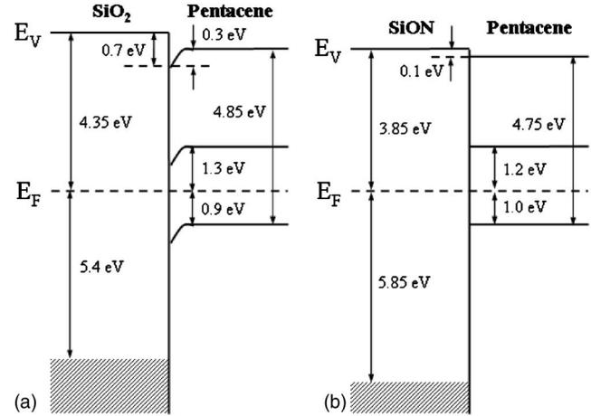
FIG. 8. Energy level diagram of pentacene on (a) the SiO<sub>2</sub> surface and on (b) the SiON surface. The magnitude of interface dipole at the pentacene/SiO<sub>2</sub> interface is larger than that at the pentacene/SiON by 0.6 eV.
