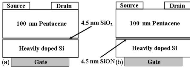
FIG. 1. Schematic device structure of the inverted-staggered pentacene thin film transistors (a) with a SiO<sub>2</sub> gate dielectric layer and (b) with a SiON gate dielectric layer.
