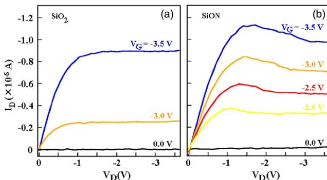
FIG. 2. (Color online) Field effect transistor characteristics of our pentacene TFTs:  $I_D$ – $V_D$  curves at various  $V_G$  obtained from TFTs with (a) the SiO<sub>2</sub> gate dielectric layer and with (b) the SiON gate dielectric layer (channel length  $L=50 \mu\text{m}$  and width  $W=1000 \mu\text{m}$ ).
