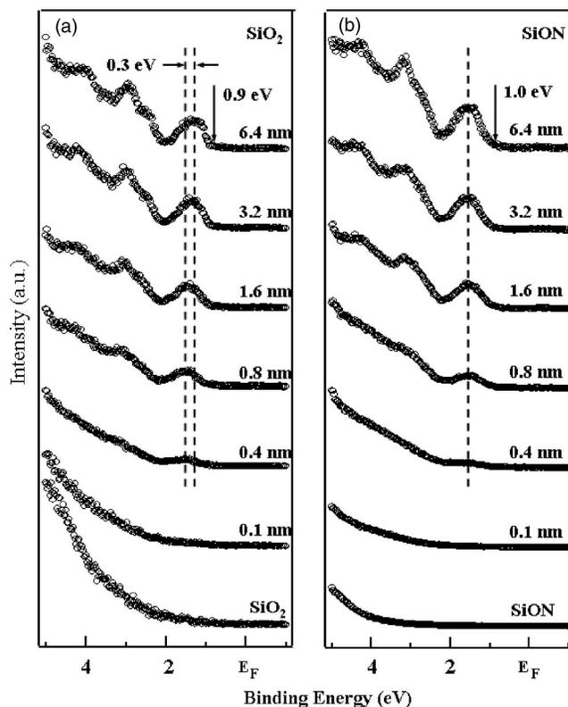
FIG. 6. The UPS spectra collected near the Fermi level as a function of pentacene deposition on (a) the SiO<sub>2</sub> surface and on (b) the SiON surface.
