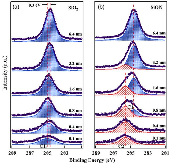
FIG. 7. (Color online) The core-level spectra of C 1s obtained during the pentacene deposition on (a) the SiO<sub>2</sub> surface and on (b) the SiON surface, respectively. Decompositions of the spectra by curve-fitting analyses are also shown, with different component marked by different shading.
