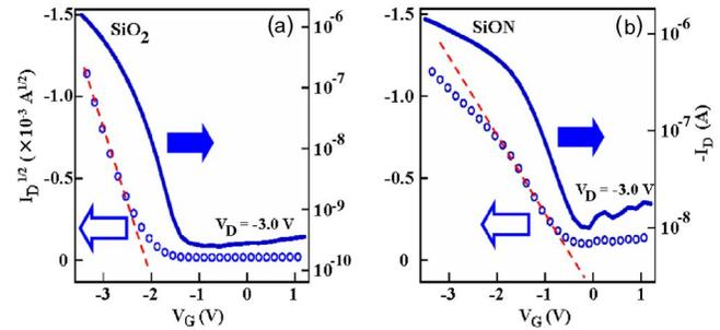
FIG. 3. (Color online) Field effect transistor characteristics of our pentacene TFTs:  $\sqrt{I_D}$ – $V_G$  curves for the estimation of saturation regime mobility that were obtained at  $V_D=-3 \text{ V}$  from TFTs with (a) the SiO<sub>2</sub> dielectric layer and with (b) the SiON dielectric layer (channel length  $L=50 \mu\text{m}$  and width  $W=1000 \mu\text{m}$ ).
