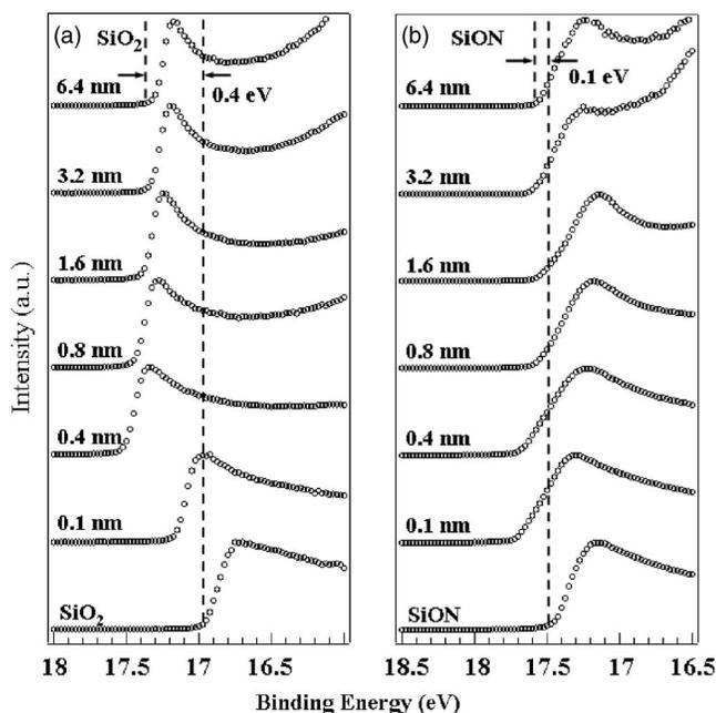
FIG. 5. The UPS spectra in the secondary cutoff region collected during the step-by-step layer deposition of pentacene on (a) the SiO<sub>2</sub> surface and on (b) the SiON surface.
