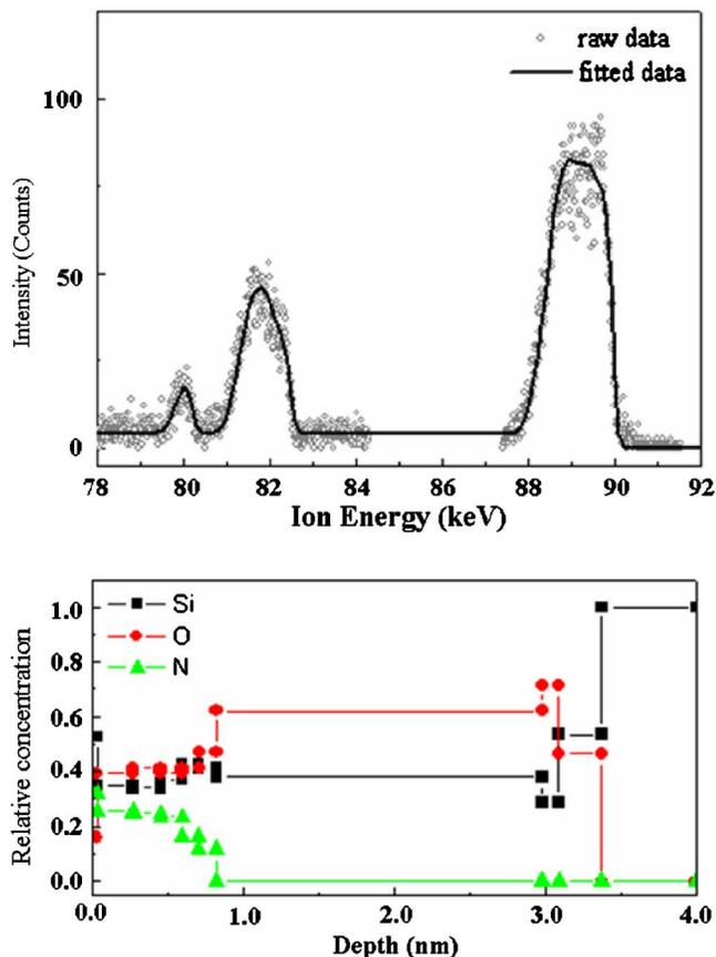
FIG. 4. (Color online) MEIS spectra of the SiON gate dielectric layer. The bottom part shows the depth-profiling data obtained from fitted MEIS spectra.
