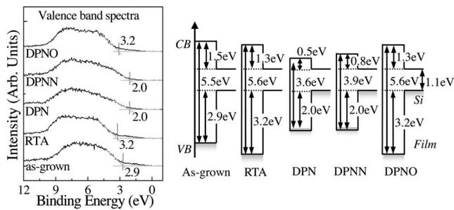
FIG. 3. Valence band spectra for the HfO<sub>2</sub> films (left side) and a band alignment diagram with Si (right side) as a function of various postannealing treatment.
