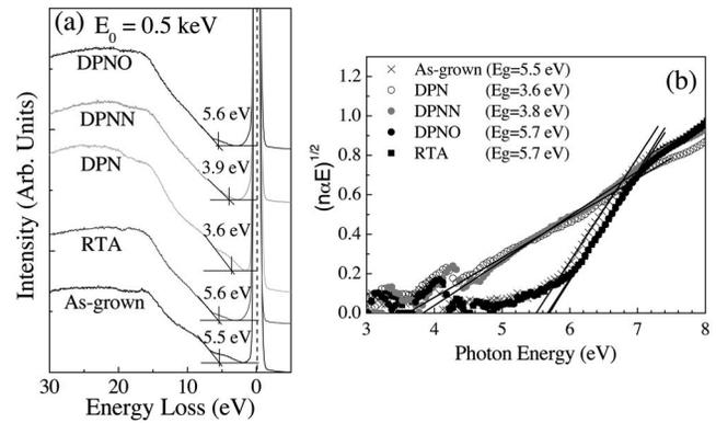
FIG. 2. Reflection electron energy loss spectra (REELS) with different electron gun energies; (a)  $E_0=0.5$  keV. Band gap using (b) spectroscopic ellipsometry is well consistent with the REELS data.
