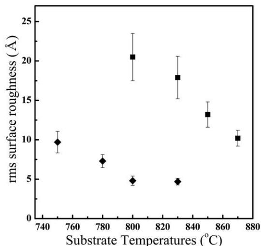
**Fig. 5** Temperature dependence of the rms surface roughness of  $\text{Al}_2\text{O}_3$  films grown on an oxidized Si surface ( $\blacklozenge$ ) and a clean Si surface ( $\blacksquare$ ).
