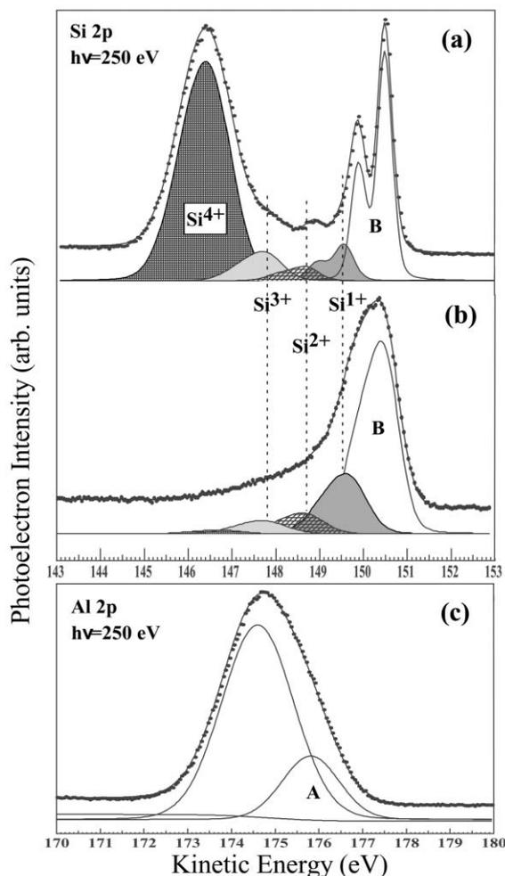
**Fig. 3** Si 2p photoelectron spectra for the oxidized Si substrate (a) before and (b) after  $\text{Al}_2\text{O}_3$  film growth. Each suboxide component is indicated by different shading. Decomposition of Al 2p spectrum is depicted in (c).
