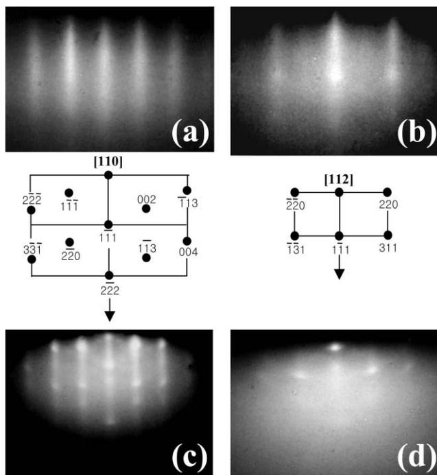
**Fig. 1** RHEED patterns along the (a)  $\langle 110 \rangle$  and (b)  $\langle 112 \rangle$  azimuth of  $\gamma\text{-Al}_2\text{O}_3$  films grown on an oxidized Si(111) substrate at a temperature of 850 °C. RHEED patterns observed along the  $\langle 110 \rangle$  azimuth of the  $\text{Al}_2\text{O}_3$  films (c) grown on an oxidized Si surface at 800 °C and (d) grown on a clean Si surface at 830 °C.
