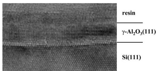
**Fig. 4** HRTEM image of epitaxial  $\text{Al}_2\text{O}_3(111)$  film grown on an oxidized Si(111) substrate at  $830^\circ\text{C}$ .
