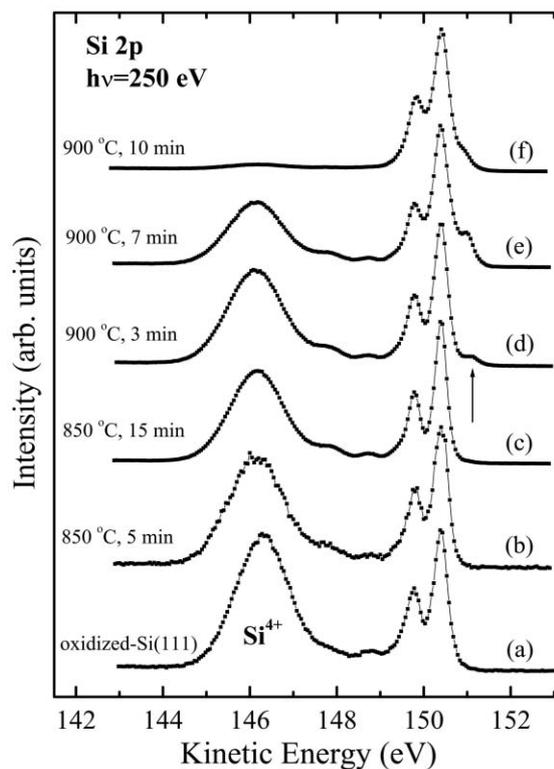
**Fig. 2** Temperature and time dependence of the oxidized Si substrate.
