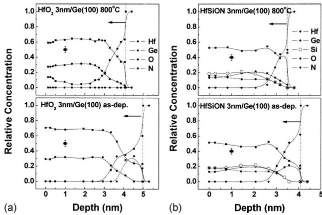
FIG. 2. Compositional depth profile obtained by simulating MEIS energy spectra for as-deposited and annealed (a)  $\text{HfO}_2$  films and (b)  $\text{HfSiON}$  films on  $\text{Ge}(100)$  substrates. Dotted line and arrow indicate the  $\text{Ge}$  substrates and the direction of the films. The point with the error bars represents the fitting errors in the depth direction and relative concentration.
