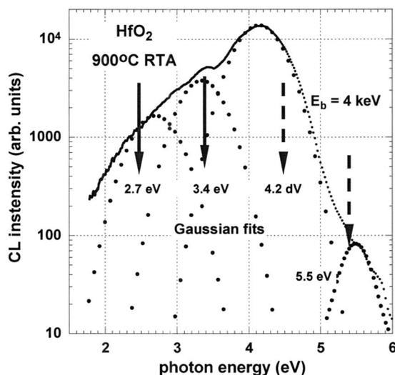
FIG. 7. Gaussian fits to four transition bands in the DRCLS for  $E_b=4\text{ keV}$  from a 100 nm thick  $\text{HfO}_2$  film a  $900^\circ\text{C}$  annealing.
