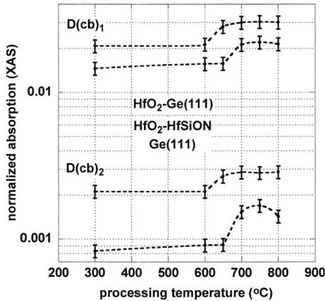
FIG. 6. Relative concentrations of defects for  $\text{HfO}_2$  on Ge(111) and stacked  $\text{HfO}_2/\text{HfSiON}$ , also on Ge(111), as function of processing temperature. The dashed lines indicate trends in the data.
