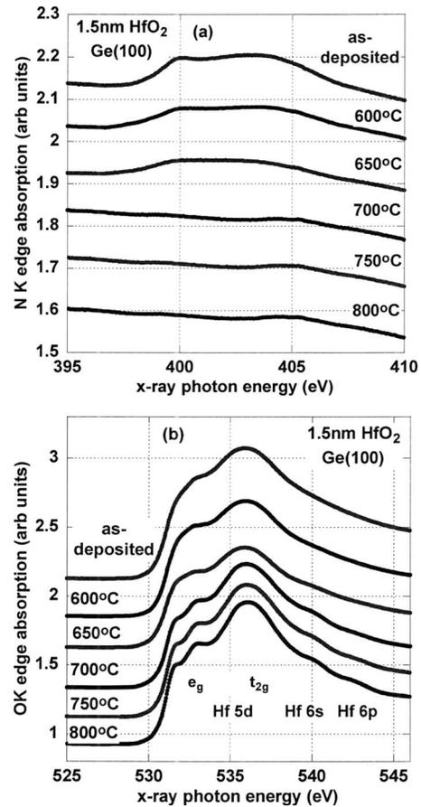
FIG. 3. (a)  $\text{N K}_1$  spectra and (b)  $\text{O K}_1$  spectra for a 1.5 nm  $\text{HfO}_2$  film on a  $\text{Ge}(100)$  substrate, as deposited at  $300^\circ\text{C}$ , and annealed to 600, 650, 700, 750, and  $800^\circ\text{C}$ .
