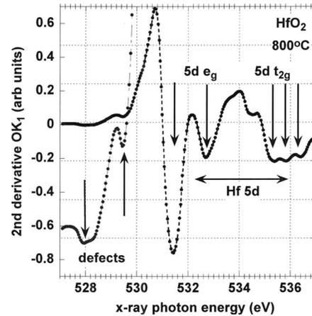
FIG. 4. Second derivative O  $K_1$  edge spectrum for a 1.5 nm thick  $\text{HfO}_2$  film on Ge(100) annealed to 800 °C, indicating Jahn-Teller split conduction band  $5d$  states, and two band edge defects in a  $10\times$  scaled insert.
