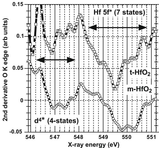
Fig. 1. Virtual bound resonances in vacuum continuum region of O K edge second derivative XAS spectra for thin film  $m$ - and  $t$ -HfO<sub>2</sub>.
