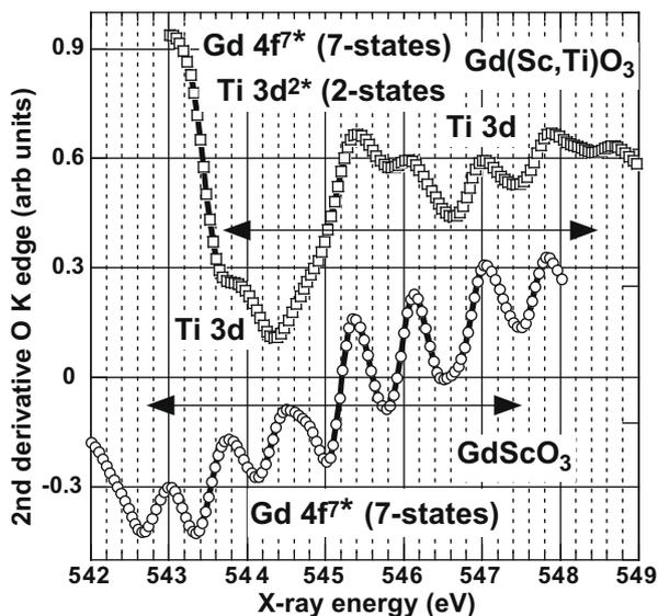
Fig. 5. Gd 4f and Ti 3d anti-bonding features in vacuum continuum region of O K edge second derivative XAS spectra for  $\text{GdScO}_3$  and  $\text{Gd}(\text{Sc}_{0.96}\text{Ti}_{0.04})\text{O}_3$ .
