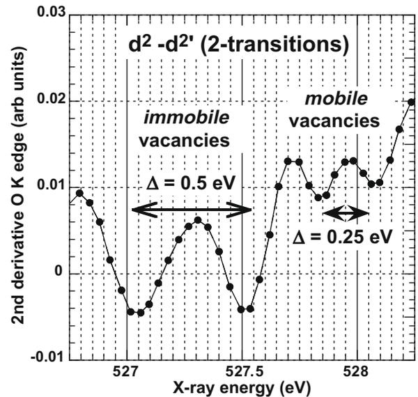
Fig. 3. Pre-edge O K edge second derivative XAS spectra for fixed and mobile vacancies in thin film TiO<sub>2</sub>.
