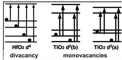
Fig. 6. Energy level diagrams proposed for d-d' transitions associated with monovacancy and divacancy  $d^2$  and  $d^4$  defects in nano-grain  $\text{TiO}_2$  and  $\text{HfO}_2$ , respectively.
