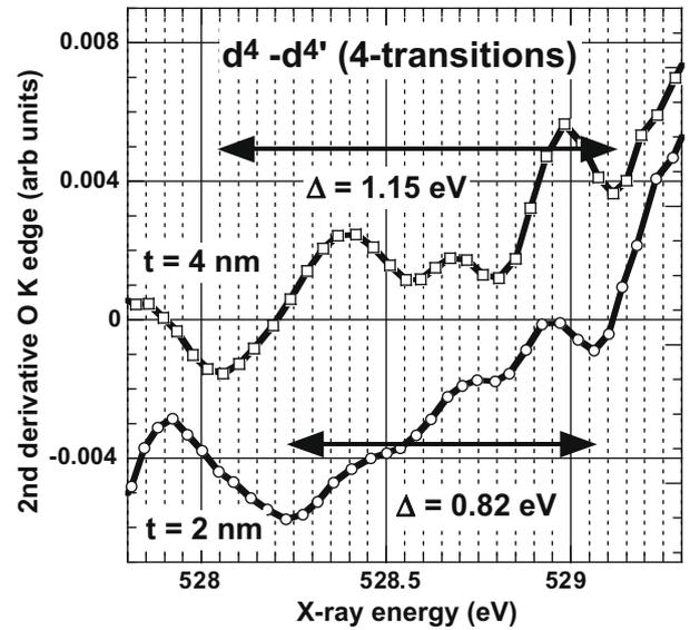
Fig. 2. Highest 5d–5d' transitions for divacancy  $d^4$  defects in the pre-edge second derivative XAS O K edge spectra for 4 nm thick and 2 nm thick HfO<sub>2</sub> thin films.
