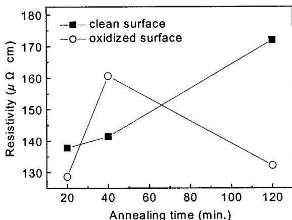
FIG. 5. Measured electrical resistivity of the Gd-silicide films grown on the clean Si surface and the oxidized Si surface as a function of annealing time.
