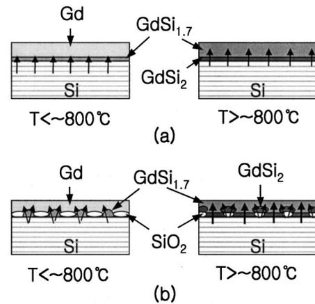
FIG. 3. The schematic diagrams representing the reaction pathway of the Gd-silicide layer via solid-state reaction in postannealing. (a) Gd-silicide film formation on the clean Si surface, (b) Gd-silicide film formation on the Si surface with interfacial  $\text{SiO}_2$  layer.
