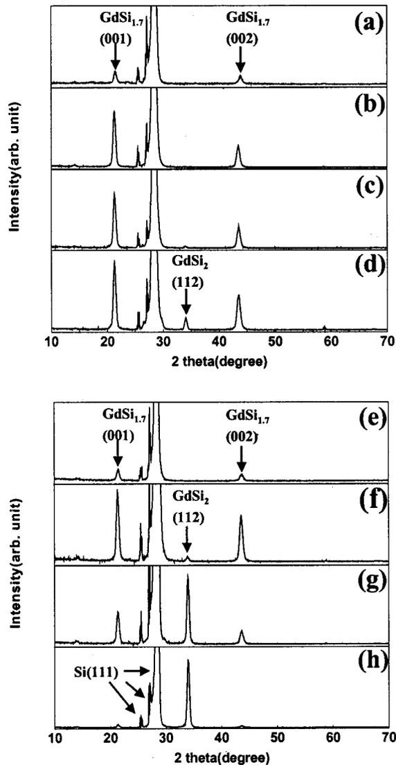
FIG. 2. XRD data collected from the sample with Gd layer on the clean Si surface after (a) deposition, annealing at 800 °C for (b) 20 min, (c) 40 min, (d) 120 min, from the sample with Gd layer on the oxidized Si surface after (e) deposition, annealing at 800 °C for (f) 20 min, (g) 40 min, (h) 120 min.
