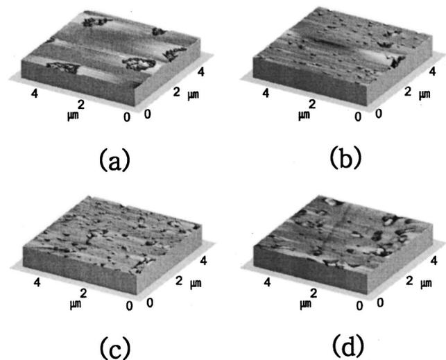
FIG. 4. AFM images collected on the sample prepared on the oxidized Si surface after (a) Gd layer deposition, annealed at 800 °C for (b) 20 min, (c) 40 min, and (d) 120 min, respectively.
