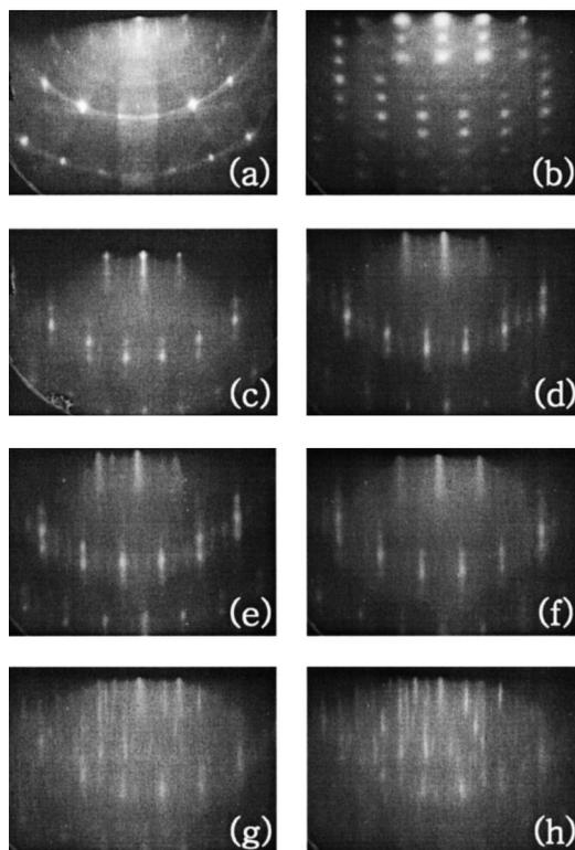
FIG. 1. RHEED patterns observed from the (a) Si(111)- $7\times 7$  surface before Gd deposition, (b) as-deposited Gd film on Si(111), Gd-silicide layer grown on the clean Si surface after annealing for (c) 20 min, (d) 40 min, (e) 120 min, Gd-silicide layer grown on the oxidized Si surface after annealing for (f) 20 min, (g) 40 min, (h) 120 min. The incident electron beam is along the  $[112]$  direction.
