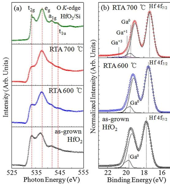
FIG. 3. (Color online) (a) NEXAFS spectra of the O  $K$ -edge features for HfO<sub>2</sub>/GaAs films. The O  $K$ -edge features of the NEXAFS spectra in the HfO<sub>2</sub> films were changed after the postannealing treatments. (b) Hf  $4f$  core-level spectra for HfO<sub>2</sub>/GaAs films were measured by XPS as a function of postannealing temperature.
