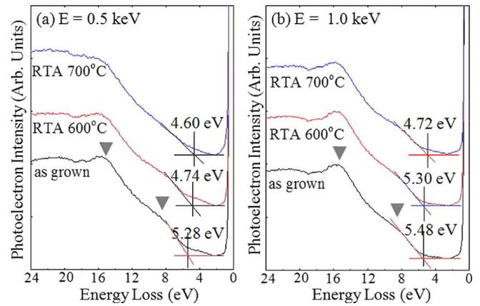
FIG. 4. (Color online) REELS spectra for HfO<sub>2</sub>/GaAs films as function of postannealing temperature, using an incident electron energy of 1.0 keV. The  $E_g$  values were defined as the threshold energy of band-to-band excitation. The arrows represent the HfO<sub>2</sub> surface plasmon peak near 9 eV and the bulk plasmon peak near 16 eV, respectively.
