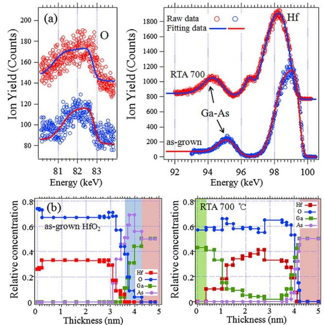
FIG. 2. (Color online) (a) Hf, Ga-As, and O peaks of measured MEIS spectra and (b) compositional depth profiles for 4-nm-thick HfO<sub>2</sub>/GaAs films as a function of postannealing temperature. The Ga and As peaks were observed as one peak, in which the Ga and As peaks are overlapped, due to the similarity of each atomic mass.
