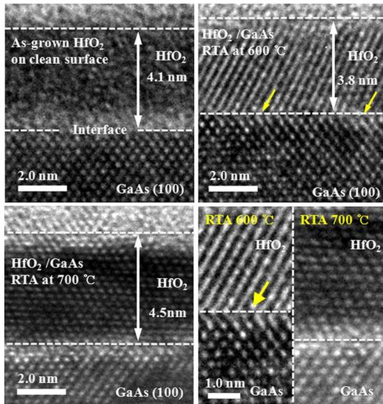
FIG. 1. (Color online) HRTEM images of HfO<sub>2</sub> films on a BOE treated GaAs (100) surface are shown along the GaAs [110] direction. The image shows changes in the crystal structure from an amorphous to a crystalline phase during postannealing processes at 600 °C. The arrows represent the lattice mismatch for interfacial atoms between the HfO<sub>2</sub> film and the GaAs substrate.
