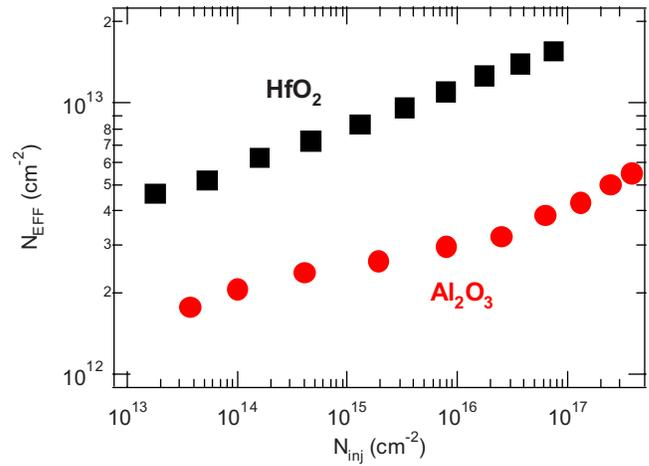
FIG. 2. (Color online) Effectively trapped charge density ( $N_{\text{eff}}$ ) determined by the flat band voltage shifts ( $\Delta V_{\text{fb}}$ ) in  $C$ - $V$  hysteresis measurements vs injected charge density ( $N_{\text{inj}}$ ) determined from the current injected during the  $C$ - $V$  sweep.
