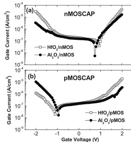
FIG. 3. Gate leakage current-voltage plots for (a) HfO<sub>2</sub> and Al<sub>2</sub>O<sub>3</sub> of  $n$ -Ge MOS capacitor and (b) HfO<sub>2</sub> and Al<sub>2</sub>O<sub>3</sub> of  $p$ -Ge MOS capacitor. The current level at the given gate voltage in this plots was used for the estimation of injected charge density ( $N_{\text{inj}}$ ) in Eq. (2).
