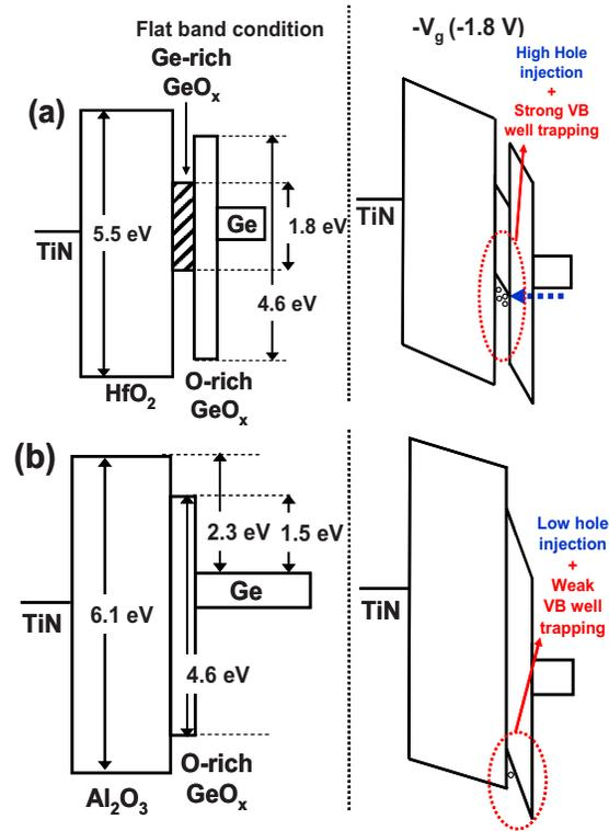
FIG. 6. (Color online) Schematic band alignment of gate stacks in  $p$ -Ge MOS capacitors for (a)  $\text{HfO}_2/\text{Ge-rich GeO}_x/\text{O-rich GeO}_x$  and (b)  $\text{Al}_2\text{O}_3/\text{O-rich GeO}_x$  interfaces.
