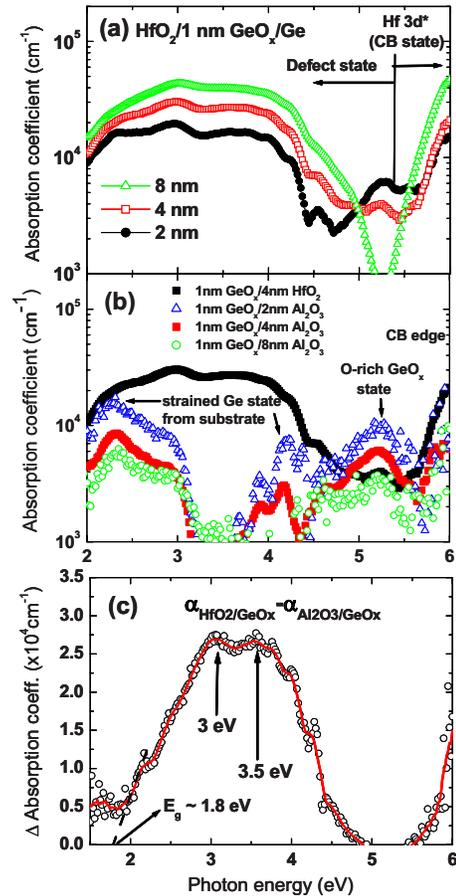
FIG. 4. (Color online) Absorption coefficient spectra from SE measurement of (a) HfO $_2$  with different thicknesses (2/4/8 nm) on 1 nm GeO $_x$  interlayer and (b) 4 nm HfO $_2$  and 2/4/8 nm Al $_2$ O $_3$  on 1 nm GeO $_x$ . (c) Differentiated absorption spectra of 4 nm HfO $_2$  with respect to 4 nm Al $_2$ O $_3$  on 1 nm GeO $_x$  as in (b).
