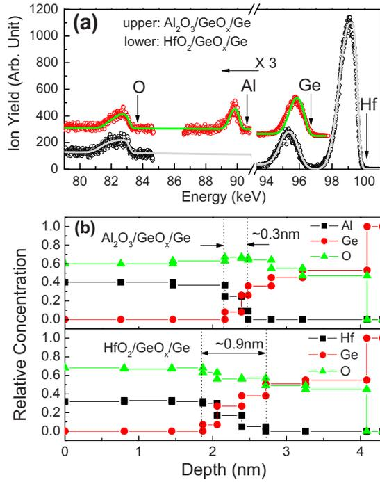
FIG. 5. (Color online) (a) MEIS energy spectra for 2 nm  $\text{HfO}_2$  and  $\text{Al}_2\text{O}_3$  on 1 nm  $\text{GeO}_x$  and (b) depth profiles constructed from a simulation of the spectra in (a).
