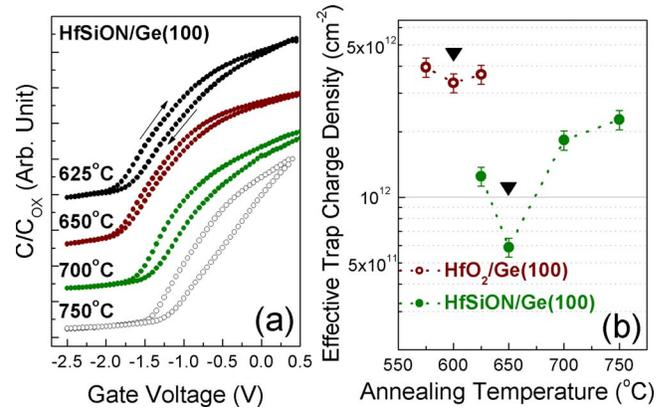
FIG. 4. (Color online) (a) CV characteristics of  $n$ -type MOS capacitor of 5 nm  $\text{HfSiON}$  on  $n$ -type  $\text{Ge}(100)$ , normalized by  $C/C_{\text{OX}}$ , as a function of PDA temperature. The arrow provides the direction of hysteresis, indicating the clockwise hysteresis loop. (b) Thermal evolution of effective trap charge density, calculated by the hysteresis offset of CV characteristics.
