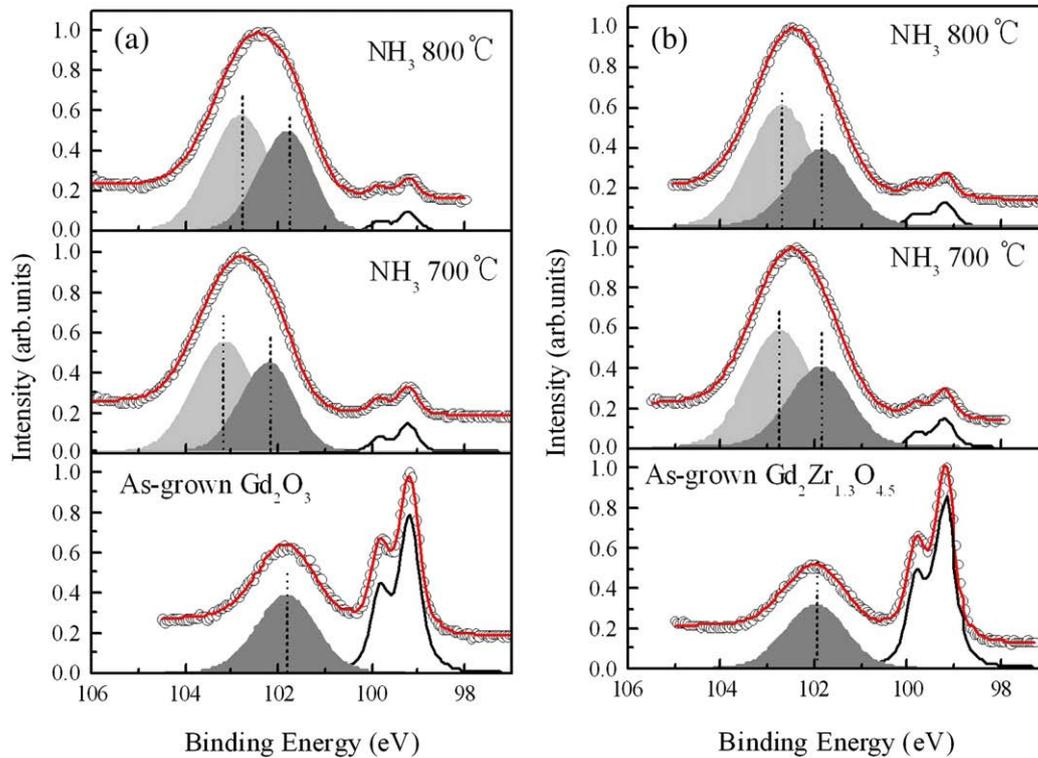
**Fig. 4.** Si 2p XPS spectra of (a) as-grown and nitrated  $\text{Gd}_2\text{O}_3$  film (2 nm) in an ambient of  $\text{NH}_3$  at 700 °C, 800 °C, and (b) as-grown and nitrated  $\text{Gd}_2\text{Zr}_{1.3}\text{O}_{4.5}$  film (2 nm) in an ambient of  $\text{NH}_3$  at 700 °C and 800 °C, respectively.
