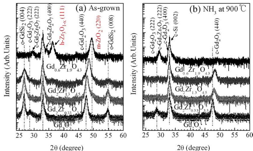
Fig. 1. XRD patterns ( $\theta$ – $2\theta$  scan) of  $Gd_2O_3$  and Zr-incorporated  $Gd_2O_3$  films (30 nm) grown on Si(100) as a function of zirconium content (a) without any nitridation process and (b) with  $NH_3$  nitridation at 900 °C. (c: cubic, m: monoclinic, h: hexagonal, and o: orthorhombic phase).
