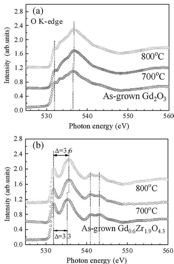
Fig. 6. Oxygen K-edge NEXAFS spectra for (a) as-grown and nitrided  $\text{Gd}_2\text{O}_3$  films (30 nm) at 700 °C, 800 °C and (b) as-grown and nitrided  $\text{Gd}_{0.6}\text{Zr}_{1.9}\text{O}_{4.3}$  films (30 nm) at 700 °C and 800 °C.
