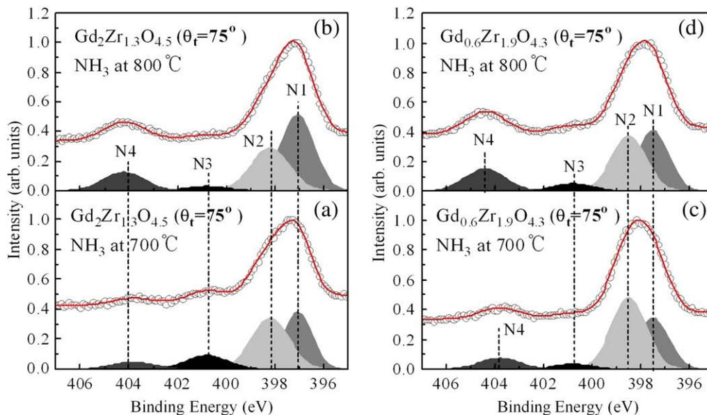
**Fig. 5.** N 1s XPS spectra (as shown in Fig 3 take-off angles 75°) of a  $\text{Gd}_2\text{Zr}_{1.3}\text{O}_{4.5}$  film nitrated in an ambient of  $\text{NH}_3$  at 700 °C (a), 800 °C (b), and a  $\text{Gd}_{0.6}\text{Zr}_{1.9}\text{O}_{4.3}$  film nitrated in an ambient of  $\text{NH}_3$  at 700 °C (c) and 800 °C (d), respectively.
