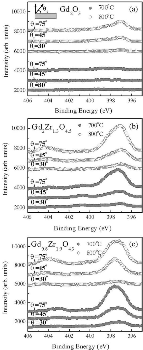
**Fig. 3.** N 1s ARXPS spectra taken at various take-off angles ( $75^\circ$ ,  $45^\circ$ , and  $30^\circ$ ) for various compositions of (a) as-grown  $\text{Gd}_2\text{O}_3$ , (b)  $\text{Gd}_2\text{Zr}_{1.3}\text{O}_{4.5}$ , and (c)  $\text{Gd}_{0.6}\text{Zr}_{1.9}\text{O}_{4.3}$  films as a function of nitridation temperature in an ambient of  $\text{NH}_3$  at  $700^\circ\text{C}$  and  $800^\circ\text{C}$ , respectively. (Thickness of each film: 4 nm).
