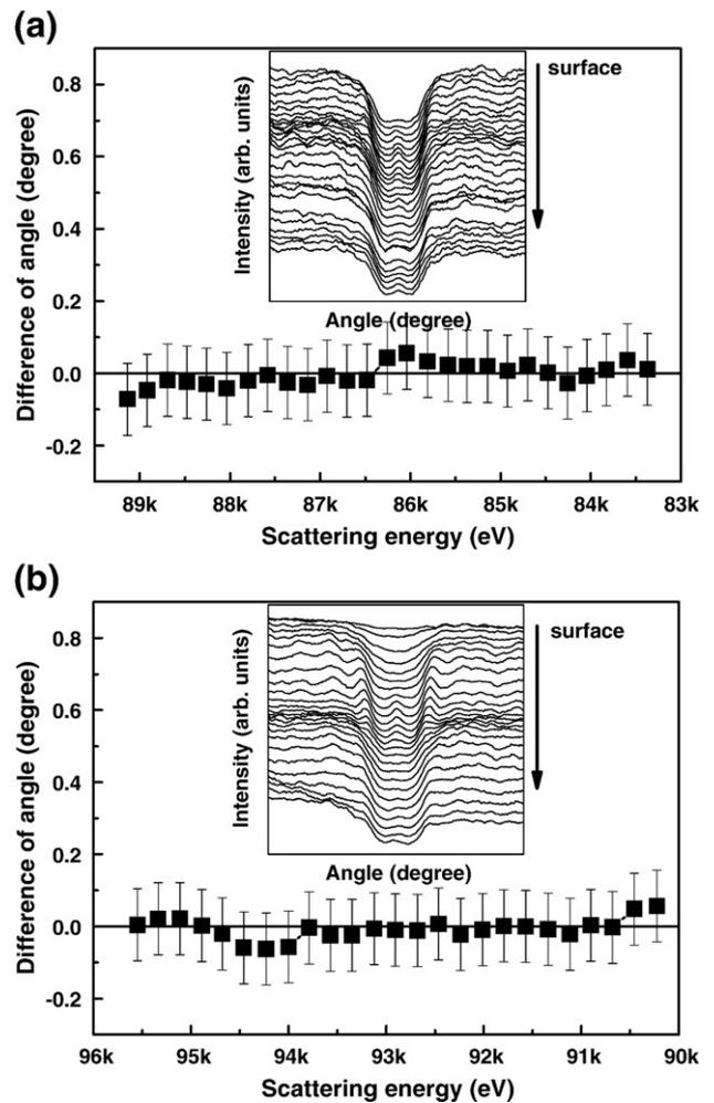
Fig. 2. Shift of the blocking dip positions of the (a) Si and (b) Ge peaks for as-deposited  $\text{Si}_{0.7}\text{Ge}_{0.3}$ .
