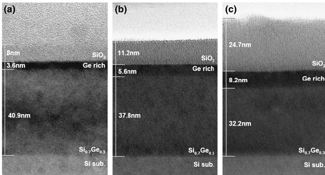
Fig. 1. TEM images of oxidized  $\text{Si}_{0.7}\text{Ge}_{0.3}$  at  $800^\circ\text{C}$  after (a) 30 min, (b) 60 min, and (c) 120 min.
