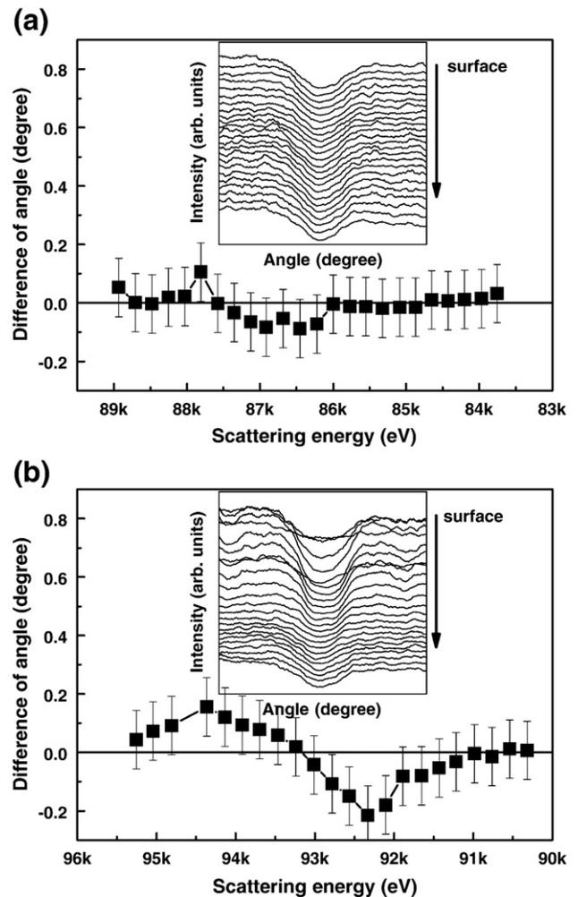
Fig. 4. Shift of the blocking dip positions of the (a) Si and (b) Ge peaks for  $\text{Si}_{0.7}\text{Ge}_{0.3}$ , which was oxidized for 120 min.
