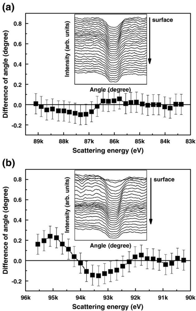
Fig. 3. Shift of the blocking dip positions of the (a) Si and (b) Ge peaks for  $\text{Si}_{0.7}\text{Ge}_{0.3}$ , which was oxidized for 30 min.
