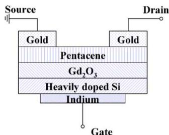
Fig. 1. Schematic diagram of pentacene TFTs used in this experiment. Top contact structure was adopted. The device had a top contact structure with a 200 nm thick pentacene layer on a 280 nm thick  $\text{Gd}_2\text{O}_3$  layer.
