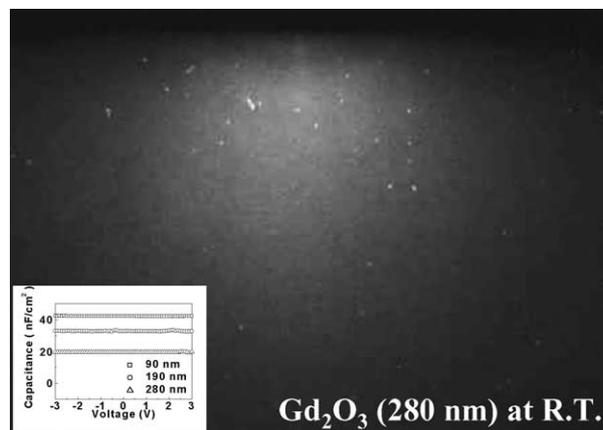
Fig. 2. The RHEED pattern, taken from the  $\text{Gd}_2\text{O}_3$ , indicates amorphous phase of the film grown on clean silicon (100) surface at room temperature. The C–V plots are shown in inset.
