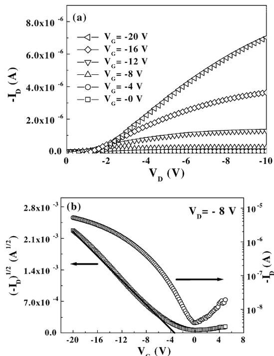
Fig. 4. (a) Drain current–drain voltage characteristics of the pentacene TFTs on a thin high- $\kappa$   $\text{Gd}_2\text{O}_3$  layer, where the channel width was 1000  $\mu\text{m}$  and the channel length was 50  $\mu\text{m}$ . (b) Drain current (right y-axis) and the square root of drain current (left y-axis) vs. gate voltage plot for the  $V_D = -8$  V.
