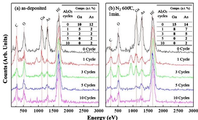
**Figure 2.** (Color online) EDS spectra of  $\text{HfO}_2/\text{Al}_2\text{O}_3/\text{GaAs}$  systems with various  $\text{Al}_2\text{O}_3$  deposition cycles: (a) as-deposited (b) after annealing at  $600^\circ\text{C}$  for 1 min in a  $\text{N}_2$  ambient.
