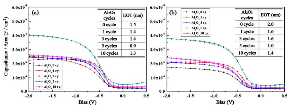
**Figure 4.** (Color online)  $C$ - $V$  characteristics at 1 MHz before (a) and after annealing (b) for  $\text{HfO}_2/\text{Al}_2\text{O}_3/\text{GaAs}$  systems using various  $\text{Al}_2\text{O}_3$  deposition cycles.
