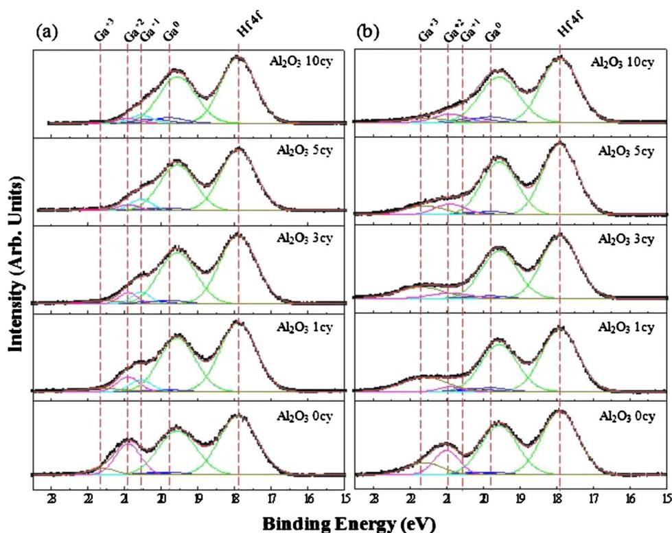
**Figure 3.** (Color online) XPS analysis results for Ga 3d spectra of  $\text{HfO}_2/\text{Al}_2\text{O}_3/\text{GaAs}$  systems with various  $\text{Al}_2\text{O}_3$  deposition cycles (a) as-deposited and (b) at  $600^\circ\text{C}$  for 1 min in a  $\text{N}_2$  ambient.
