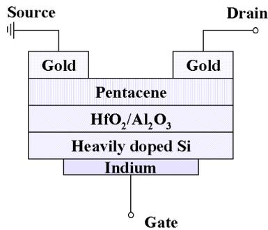
Fig. 1. Schematic diagram of the pentacene TFTs used in this experiment. The device had a top contact structure with a 100-nm-thick pentacene layer on a 3-nm thin  $\text{HfO}_2/\text{Al}_2\text{O}_3$  layer.
