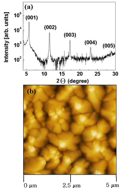
Fig. 3. (a) X-ray diffraction pattern taken from the pentacene layer on a  $\text{HfO}_2/\text{Al}_2\text{O}_3$  layer. (b) The AFM image of the pentacene film on a  $\text{HfO}_2/\text{Al}_2\text{O}_3$  gate oxide layer.
