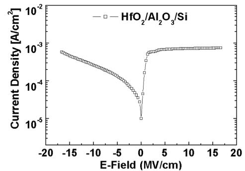
Fig. 2. Plot of the current density versus electric field for the  $\text{Au}/\text{HfO}_2/\text{Al}_2\text{O}_3/\text{Si}$  (heavily doped) structure.
