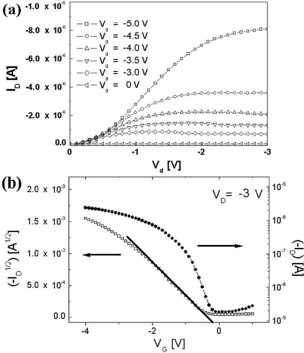
Fig. 4. (a) Drain current-drain voltage characteristics of the pentacene TFTs on thin  $\text{HfO}_2/\text{Al}_2\text{O}_3$  layers, where the channel width was  $1000 \mu\text{m}$  and the channel length was  $50 \mu\text{m}$ . (b) Drain current (right  $y$ -axis) and the square root of the drain current (left  $y$ -axis) vs. gate voltage for  $V_D = -3$  V.
