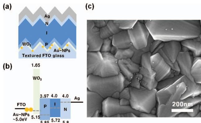
**Figure 1.** (a) Schematic device structure and (b) band diagram of solar cells with various buffer layers, including a Au-NP / WO<sub>3</sub> double buffer layer, (c) UHR FE-SEM image of spin-coated (2000 rpm) Au-NPs (~10 nm) on textured FTO glass.
