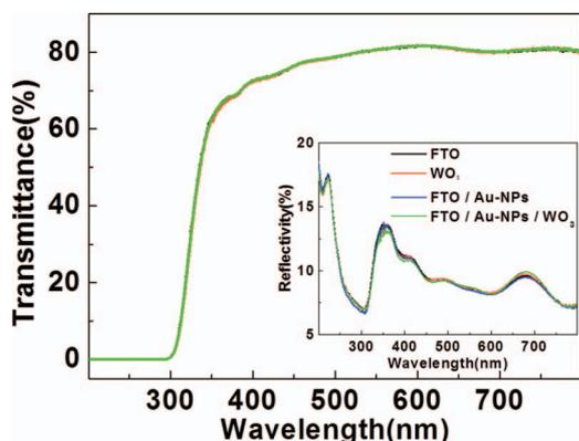
**Figure 3.** The transmittance of a textured FTO glass with a  $\text{WO}_3$  single buffer layer, Au-NP single buffer layer, and a Au-NP /  $\text{WO}_3$  double buffer layer. The inset shows the reflectivity data.
