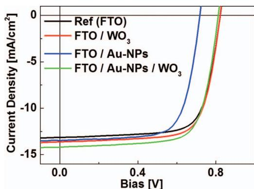
**Figure 2.** The  $J$ - $V$  characteristics ( $J_{sc}$ ) of solar cells with various buffer layers, including a  $\text{WO}_3$  single buffer layer, a Au-NP single buffer layer, and a Au-NP /  $\text{WO}_3$  double buffer layer.
