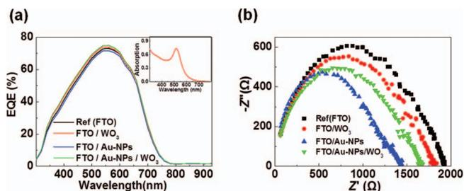
**Figure 4.** (a) The EQE and (b) impedance data of devices with a  $\text{WO}_3$  single buffer layer, a Au-NP single buffer layer, and a Au-NP /  $\text{WO}_3$  double buffer layer. The inset in (a) shows the absorption data of Au-NPs (10 nm) in solution.
