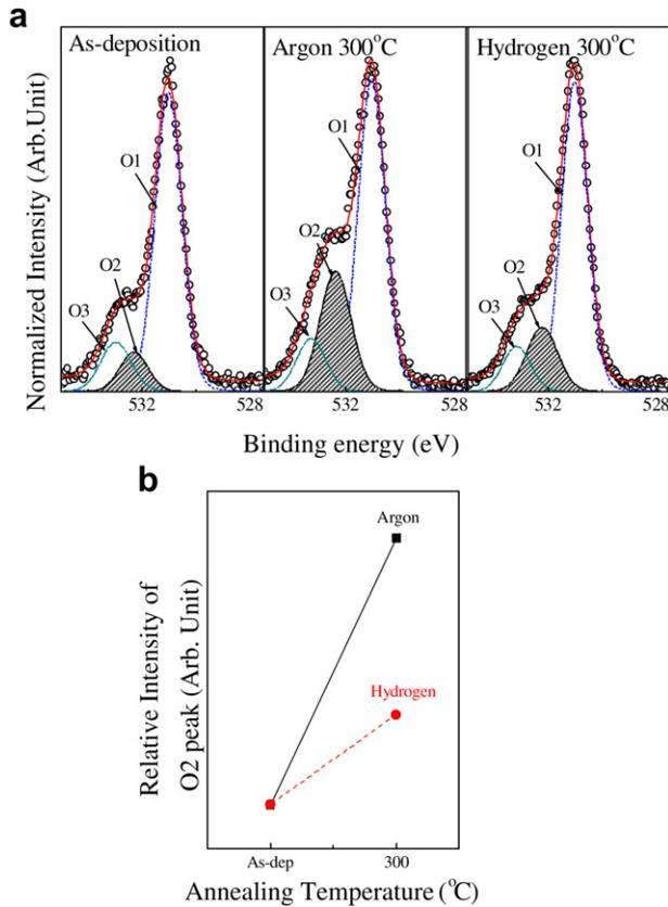
**Fig. 3.** (a) XPS spectra of O 1s for as-deposited and annealed ZnO films in the ambient atmospheres of Ar or hydrogen gas at 300 °C. Spectra were deconvoluted into the detailed O1, O2, and O3 states. (b) Relative intensity of O2 state (oxygen vacancies) for as-deposited and annealed ZnO films in the ambient atmospheres of Ar or hydrogen gas at 300 °C.
