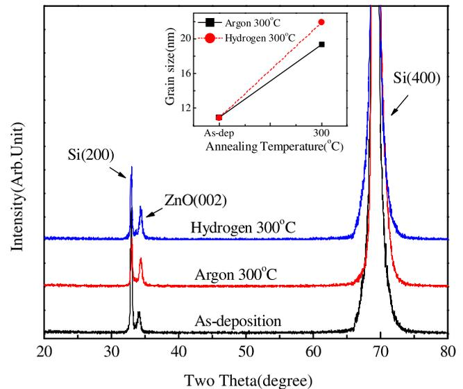
**Fig. 2.** XRD data collected from the as-deposited and annealed ZnO films in the ambient atmospheres of Ar or hydrogen gas at 300 °C. Inset is the calculated results for grain size.
