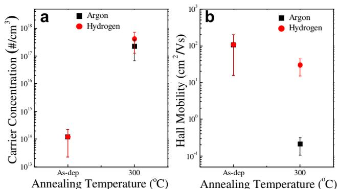
**Fig. 1.** (a) Carrier concentration and (b) hall mobility of the as-deposited and annealed ZnO films in the ambient atmospheres of Ar or hydrogen gas at 300 °C.
