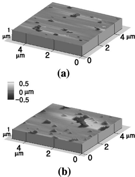
Fig. 3. AFM images collected on the samples prepared on the oxidized Si surface after the 1 h post-annealing at (a) 600 °C and (b) 900 °C, respectively.
