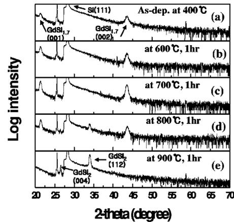
FIG. 2. XRD data collected with theta-2theta x-ray diffractometer from the samples after each indicated annealing steps.
