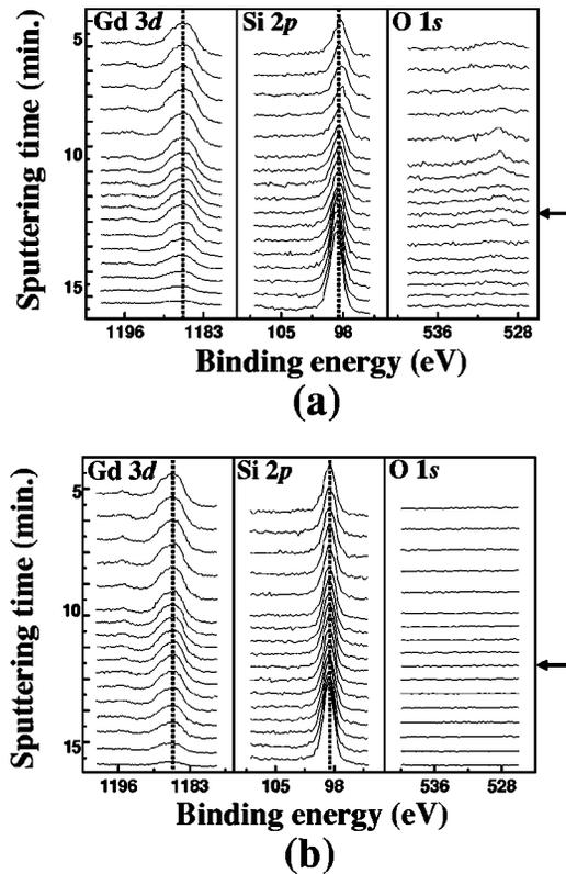
Fig. 4. XPS depth profiling spectrum taken near the interface between Gd metal and Si substrate of each samples after annealing at (a) 600 °C and (b) 900 °C, respectively.
