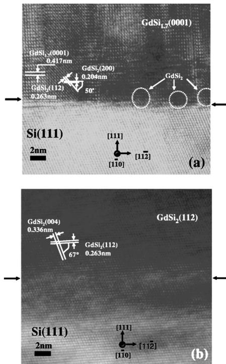
FIG. 5. HRTEM images of the samples on the oxidized Si(111) surface after (a) as-deposition at 400 °C, and (b) post-annealing at 900 °C for 1 h. The location of interface between Gd-silicide layer and Si(111) substrate is indicated by arrows in each image.
