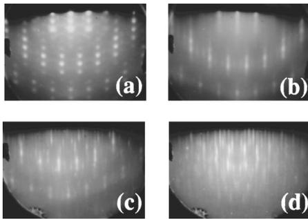
FIG. 1. RHEED patterns taken from the Gd-silicide layer grown on the oxidized Si(111) surface with the incident beam along the [112] direction after the 1 h annealing at (a) 600 °C, (b) 700 °C, (c) 800 °C, and (d) 900 °C, respectively.
