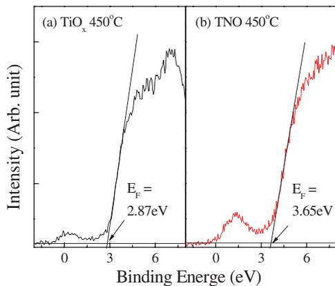
**Figure 4.** Valence band offsets measured by XPS analyses for the (a)  $\text{TiO}_x$  and (b) TNO films annealed at  $450^\circ\text{C}$ . A peak associated with sub-gap defects appears in the spectrum taken from the TNO film.
