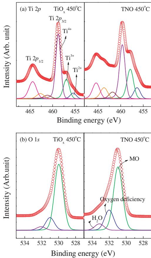
**Figure 3.** XPS peaks of (a) the titanium 2p orbitals from  $\text{TiO}_x$  and TNO film, and (b) the oxygen 1s orbitals from  $\text{TiO}_x$  and TNO film annealed at  $450^\circ\text{C}$ . The main peaks are delineated in red, which are deconvoluted into sub-peaks.
