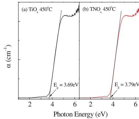
**Figure 5.** Absorption coefficient measured by SE for the (a)  $\text{TiO}_x$  and (b) film annealed at  $450^\circ\text{C}$ . The TNO film exhibits a slightly larger optical bandgap.
