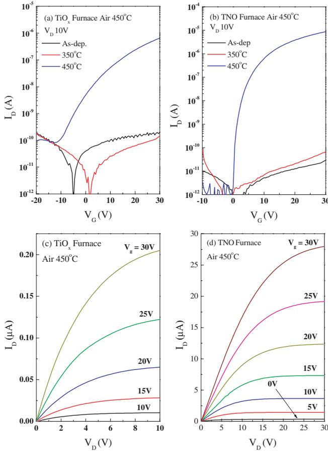
**Figure 7.** Transfer characteristics of the (a)  $\text{TiO}_x$  and (b) TNO devices. Output characteristics of the (c)  $\text{TiO}_x$  and (d) TNO devices.
