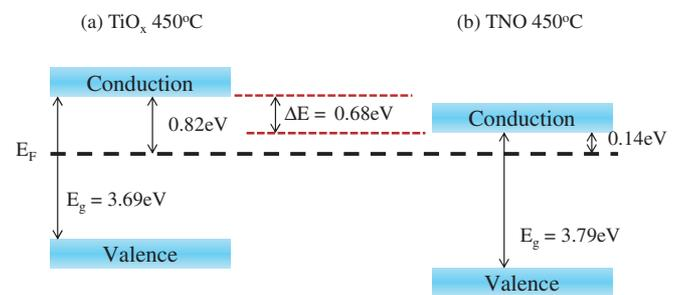
**Figure 6.** Schematic diagram of the relative position of the bandgaps between the (a)  $\text{TiO}_x$  and (b) TNO films annealed at  $450^\circ\text{C}$ .
