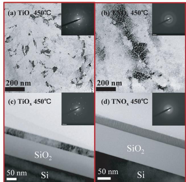
**Figure 2.** Plan-view TEM images of the (a)  $\text{TiO}_x$  film and (b) TNO film annealed at 450 °C. Cross-sectional TEM images of the (c)  $\text{TiO}_x$  film and (d) TNO film annealed at 450 °C.
