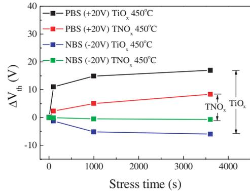
**Figure 8.** Evolution of the threshold voltage in the  $\text{TiO}_x$  and TNO devices with respect to bias stress time.
