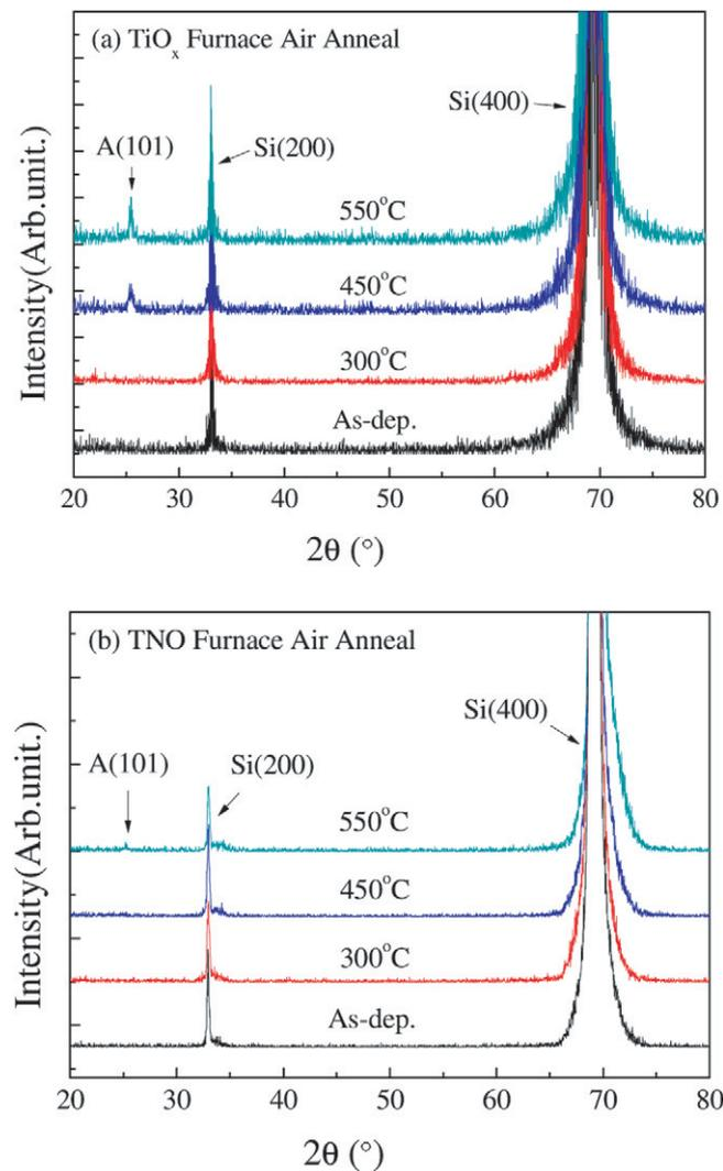
**Figure 1.** XRD patterns for the (a)  $\text{TiO}_x$  and (b) TNO films, in the as-deposited state and after heat treatment in air at different temperatures.
